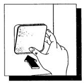
Open the panel covering the filter and place a container underneath to catch any spillage.
