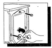
Using a spanner unscrew and remove the rear right screw.
