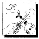
Remove and clean the filters using a hard bristle brush.
