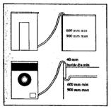
Important: Before connecting up the machine to new pipework or to pipework that has not been used for some time, run off a reasonable amount of water to flush out any debris that may have collected in the pipes.
