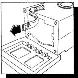
Plug the 3 holes with the 3 plastic plugs which you can find on the back of the machine.
