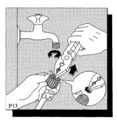
Remove and clean the filters using a hard bristle brush.
