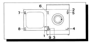
Reassemble the door closure (7) and stud (8) by reversing their position, then press thoroughly until hooking the tongue.
