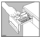
Pull out the detergent dispenser drawer from the control panel. Measure out the amount of detergent required and pour into the main wash compartment.
