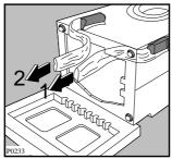
Remove the polystyrene block from the bottom of the machine
