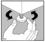
Level the washing machine by raising or lowering the feet. The feet may be tight to adjust as they incorporate a self locking nut, but the machine MUST be level.
