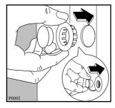
Slide out the 3 plastic spacers and plug the 3 holes with the 3 plastic plugs which you can find at the back of the machine.
