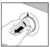
Pull the programme selector dial outwards: the mains-on light illuminates and the machine starts operating.
