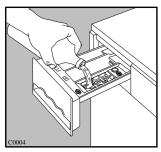
Pour the fabric softener, if required, into the compartment marked 88.
