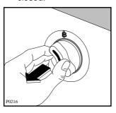
Pull the programme selector dial outwards: the mains-on light illuminates and the machine starts operating.
