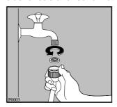
Before connecting the hoses be sure to fit the mesh filters supplied as per diagram.
