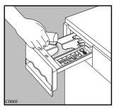
Pull out the detergent dispenser drawer from the control panel. Measure out the amount of detergent required and pour into the main wash compartment.
