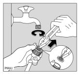
Remove and clean the filters using a hard bristle brush. Replace the filters and tighten up the inlet hoses.
