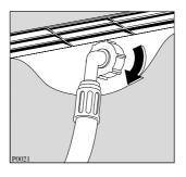
Set the hoses correctly by loosening the ring nuts. After positioning the inlet hoses, be sure to tighten the ring nuts again to prevent leaks.
