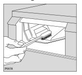
Having removed the drawer, use a small brush to clean the recess, ensuring that all washing powder residue is removed from the upper and lower part of the recess.
