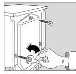
Remove the polystyrene base, set the machine upright and unscrew the two remaining rear bolts.
