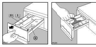
Pull out the detergent dispenser drawer from the control panel. Measure out the amount of detergent required and pour into the main wash compartment.
