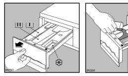
Pull out the detergent dispenser drawer from the control panel. Measure out the amount of detergent required and pour into the main wash compartment.
