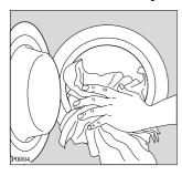
Open the door by pulling the catch outward. Load the items one at a time and close the door.
