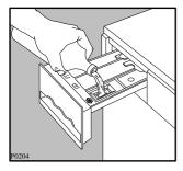
Pour the fabric softener, if required, into the compartment marked  $\bigotimes$ .
