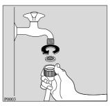
Before connecting the hoses be sure to fit the mesh filters supplied as per diagram.
