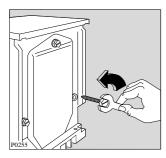
Using a spanner unscrew and remove the rear right bolt. Lay the machine gently on its back, making sure that the hoses are not squashed.
