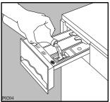
Pour the fabric softener, if required, into the compartment marked  $\bigotimes$  .
