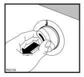
Pull the programme selector dial outwards: the mains-on light illuminates and the machine starts operating.
