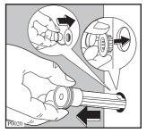
The appliance has two inlet hoses, hot and cold, with female 3/4" BSP thread connectors. If this connection is not compatible with the plumbing of the existing installation, a variety of connectors are available from good hardware stores and plumbers merchants to suit most domestic plumbing. Any alteration to your existing plumbing must be carried out by a competent person, or qualified plumber.
