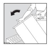
Carefully remove the polyethylene bags located at the base of the machine by pulling them toward the centre of the machine.
