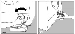
Clean the filter under a running tap, then refit it, screwing it fully in.
