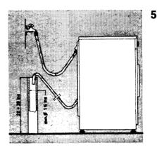
water should be able to drain freely, and the end of the outlet hose must not be under water. If a drain pipe is used, it must have an internal diameter of at least 1,5". Be sure that the drain hose is not kinked or placed in such a way as to obstruct the flow of water.
