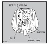
The wire coloured green and yellow must be connected to the terminal marked with the letter «E» or by the earth symbol  $\stackrel{\text{\tiny L}}{=}$  or coloured green and yellow.
