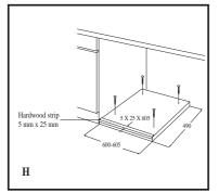
With the appliance installed adjust all four feet ensuring the machine is stable, and a clearance of approximately 5 mm is left between the top of the machine and the underside of the worktop.
