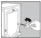
Remove the polystyrene base and take off the bottom panel by unscrewing the central screw. Carefully slide out the right polythene bag.
