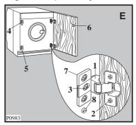
**Important:** the plastic screw (8) should **never** be loosened (Fig. B and E).
