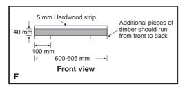
Drill four fixing holes see Fig. G
