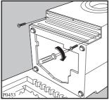
Set the machine upright and remove the two remaining bolts from the back.
