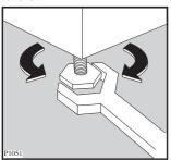
Any necessary adjustment can be made with a spanner. Accurate levelling prevents vibration, noise and displacement of the machine during operation. Some vibration is inevitable, especially if mounted on a wooden floor. Sprung wooden floors are particularly susceptible to vibration. For advice, consult a builder. If possible, always place the machine on a solid floor.
