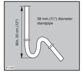
When discharging into a standpipe ensure that the top of the curve in the hose end is no more than 90cm (35.4") and no less than 60cm (23.6") above floor level.
