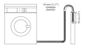
The standpipe should have an internal diameter of approximately 38mm (see diagram) thus ensuring there is an air break between the drain hose and standpipe.
