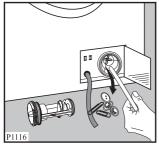
• Put the cap back on the emergency emptying hose and place the latter back in its seat.
