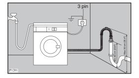
The drain hose may be extended to a maximum of 4 metres. An additional drain hose and joining piece is available from your local Service Force Centre. The joining piece must have an internal diameter of 18mm.
