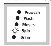
To select **Drain** only, press the "**Skip**" button three times, the **wash - rinses - spin** LED,s go out. The **Drain** LED only remains alight.
