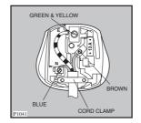
The wire coloured green and yellow must be connected to the terminal marked with the letter  $\langle E \rangle$  or by the earth symbol  $\frac{1}{2}$  or coloured green and yellow.
