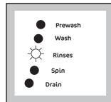
To select **Drain** the programme must be paused, now press the Skip button three times, the **wash - rinses - spin** LED,s go out.
