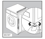
Any necessary adjustment can be made with a spanner. Accurate levelling prevents vibration, noise and displacement of the machine during operation. Some vibration is inevitable, especially if mounted on a wooden floor.
