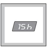
The delay time is displayed for 3 seconds, then the duration of the selected programme reappears. After you have pressed the "**Start/Pause**" button, the delay time value displayed will decrease by units of one hour every hour. When only two hours remain, the display will decrease in 30 minute steps down to zero.
