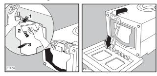
Repeat the operation for the right polythene bag, removing it towards the left and then upwards.
