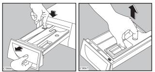
Remove the drawer by pressing the catch downwards and by pulling it out.
