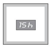
The delay time is displayed for 3 seconds, then the duration of the selected programme reappears. After you have pressed the "**Start/Pause**" button, the countdown begins, and the delay time value decreases by one unit every hour and then, when 2 hours remain, the time decreases in 30 minute intervals. You can delay the start of the selected programme by up to 23 hours in one hour intervals.
