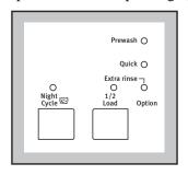
If you select the "Night Cycle" option, the machine will stop at the end of the programme with the water still in the tub.
