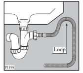
The drain hose may be extended to a maximum of 4 metres. An additional drain hose and joining piece is available from your local Service Force Centre. The joining piece must have an internal diameter of 18mm.
