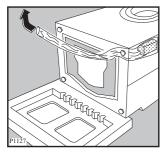
Remove the polystyrene base. Set the machine upright and unscrew the remaining rear screw. Slide out the relevant pin.
