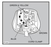
The wire coloured green and yellow must be connected to the terminal marked with the letter  $\langle E \rangle$  or by the earth symbol  $\frac{1}{2}$  or coloured green and yellow.
