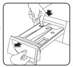
Flush it out under a tap, to remove any traces of accumulated powder.
