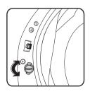
To **disable** this device and restore the possibility of closing the door, rotate the button anti-clockwise until the groove is vertical.
