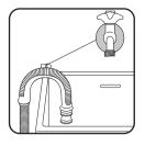
This could be done by tying it to the tap with a piece of string or attaching it to the wall.
