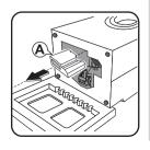
Very carefully remove the front polystyrene block
