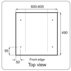
Drill four fixing holes see Fig. G
