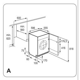
When installing the appliance into the kitchen furniture ensure, if possible, the hoses are placed in either of the two recesses on the back of the appliance.
