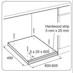
Fix the base firmly to the floor using four appropriate countersunk screws (see Fig. H).
