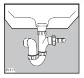
Push the drain hose onto the spigot and secure with a clip if required, ensure a loop is formed in the drain hose (see diagram) to prevent waste from the sink entering the washing machine.
