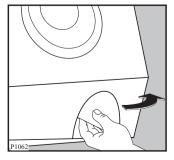
Release the emergency emptying hose, place it in the container, and remove its cap by unscrewing it.
