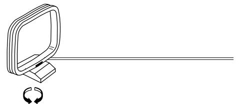
AM loop antenna
