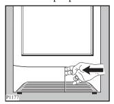
To pull out the condenser, first turn the two red stops inwards as shown and then remove the condenser unit holding it at the handle.
