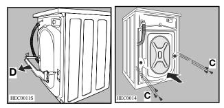
• Open the porthole and remove the polystyrene block fitted with the adhesive tape on the door seal.
