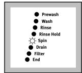
To select **Drain** only, press the "**Skip**" button three times, the **Wash - Rinse - Spin** LED,s go out. The **Drain** LED only remains alight.
