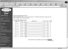
following screen to specify the additional public ports to be opened for each application. Specify the port normally associated with an application in the "Trigger Port" field, select the protocol type as TCP or UDP, then enter the public ports associated with the trigger port to open them for inbound traffic.
