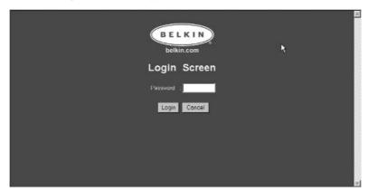
If this is the first time you are accessing the Router or you have not set a password for the Wireless Gateway Router, there is no need to enter a password. Click "Login".
