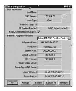
7. This window will provide you with the Adapter Address (also known as the MAC address), the IP Address, Host name (if any) and other network settings. Carefully write this information in the table below, as you may need it later for setting up the Router. For further explanation of what these setting are, see the Glossary of Network Terms in the Appendix of this manual.
