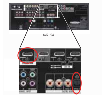
Figure 26 – Connecting an HDMI-Equipped Set-Top Box
