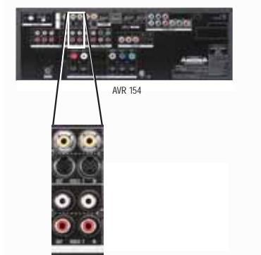
Figure 25 – Connecting a Video Recorder
