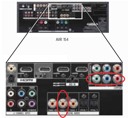
Figure 21 – Connecting a Component-Video-Equipped Disc Player
