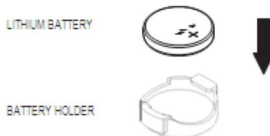
Figure 4-1. Installing the Onboard Battery
