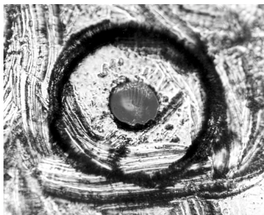
Figure 4-7. Damage from improper cleaning.
