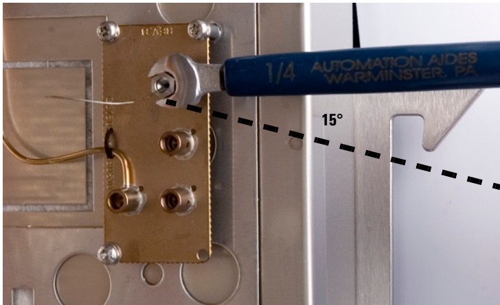
Figure 16 Tightening the connections
