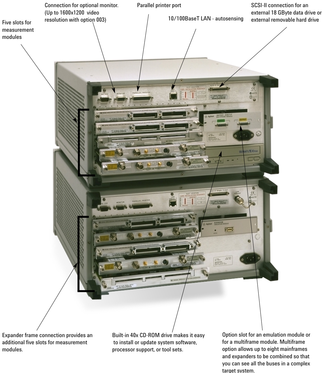
Figure 2.2. The mainframe and expander frame provide advanced capabilities for debugging complex target systems.
