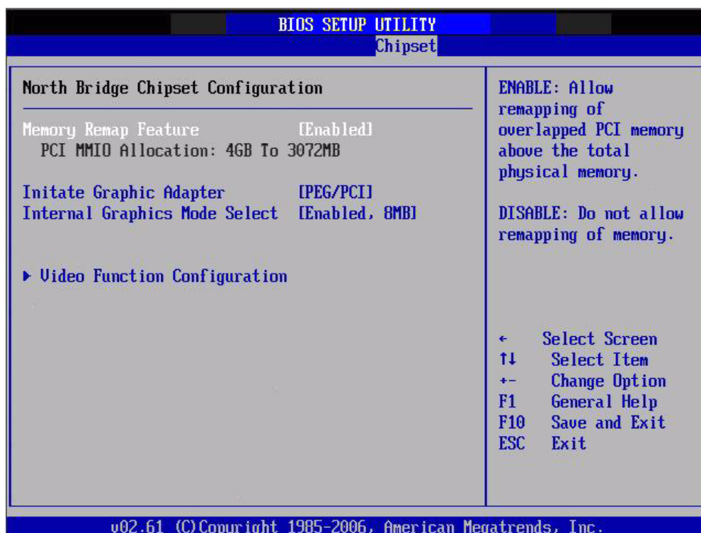
Figure 3.21 North Bridge Configuration
