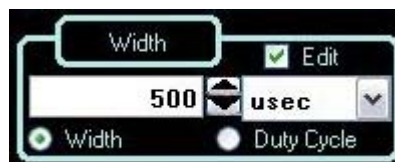
Figure 2-13 Panel view of the pulse width section
