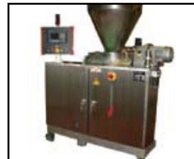
Machine Mounted Electrical Enclosure & Operator Controls
