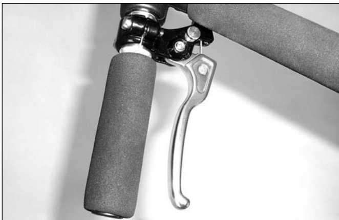
Brake lever in the parked position
