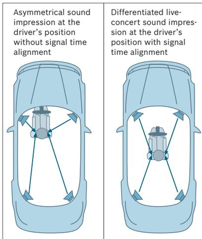
Electronically corrects the asymmetrical seating position in the vehicle by delaying the music channels so that the sound waves emitted by all the speakers reach the listener at the same time. The signal time for the Bremen MP74 can be adjusted right down to the last centimetre. It is possible to select different seating positions.
