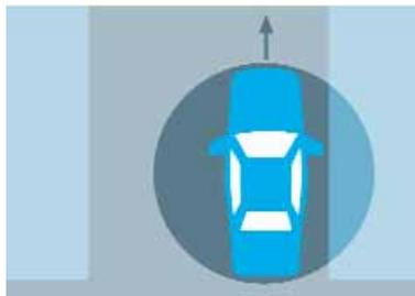
3. Now the vehicle position has been determined accurately and is updated constantly, whereby the system compares all the sensor data with the information on the digital map.
