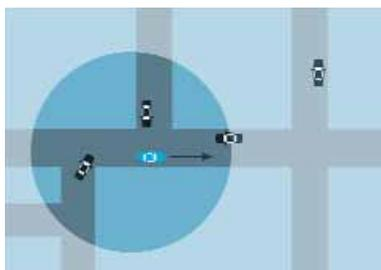
1. The GPS system makes the initial rough estimate of the vehicle location.
