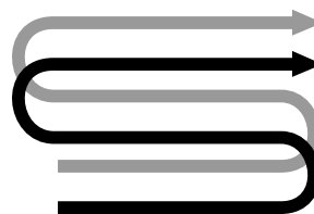
Figure 10: Use an overlap technique on every pass.
