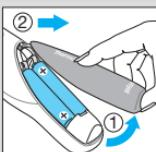
Open the battery compartment. Remove the batteries and replace with new batteries, making sure the poles are in the right direction.
