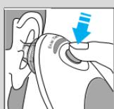
1. To achieve accurate readings, make sure a new, clean lens filter (1) is in place before each measurement.
