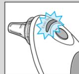
4. If the probe has not been constantly placed in a stable position in the ear canal, a sequence of short beeps will sound, the «ExacTemp» light will go out and the display will show an error message («POS» = position error).
