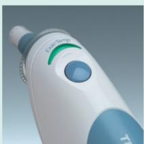
If you take the temperature of another person, the «ExacTemp» light can be of help. It flashes during the measuring process as long as the probe is securely positioned, and lights up continuously when an accurate reading has been taken.
