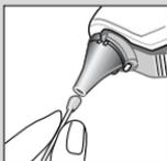
To clean the window, gently wipe its surface with a cotton swab slightly moistened with alcohol and immediately wipe dry with a clean cotton swab. After cleaning, allow at least 5 minutes drying time before taking temperatures. Make sure probe window is clean and dry. Avoid touching the window except when cleaning is required. If the window is damaged, the thermometer must be returned to Welch Allyn for service.
