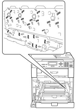
Hold the green handles of the drum unit when you carry it. DO NOT hold the side of the drum unit.  To avoid print quality problems, DO NOT touch the shaded parts shown in the illustrations.
