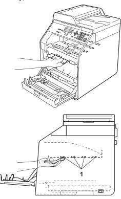
6 Make sure the green lock lever (1) is in the release position as shown in the illustration.
