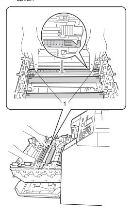
6 Clean the corona wire inside the drum unit by gently sliding the green tab from left to right and right to left several times.
