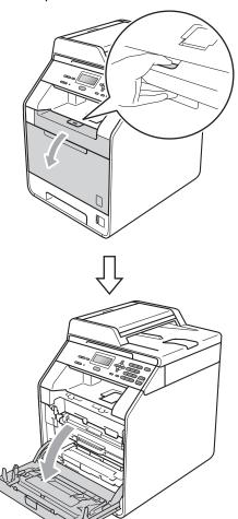
2 Hold the green handle of the drum unit. Pull the drum unit out until it stops.
