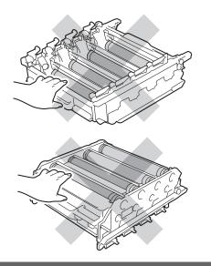
black Hold the green handle of the belt unit with both hands and lift the belt unit up, then pull it out.
