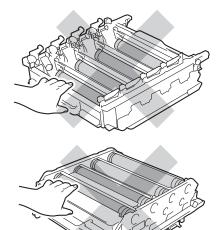
Unpack the drum unit just before you put it in the machine. Exposure to direct sunlight or room light may damage the drum unit. 7 Hold the handle of the toner cartridge and slide the toner cartridge into the new unit, then slightly pull it toward you until you hear it click into place. Make sure that you match the toner cartridge colour to the same colour label on the drum unit. Repeat this for all the toner cartridges.
