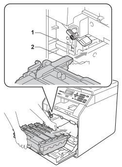
8 Turn the green lock lever (1) clockwise to the lock position.
