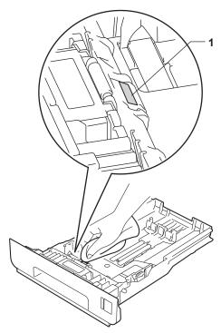
Wipe the two pick-up rollers (1) inside the machine to remove dust.
