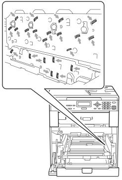
Hold the green handles of the drum unit when you carry it. DO NOT hold the side of the drum unit. 5 Pull out the jammed paper slowly.
