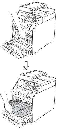
5 Turn the green lock lever (1) at the left of the machine anticlockwise to the release position. Holding the green handles of the drum unit, lift the front of the drum unit and remove it from the machine.
