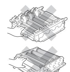
7 Turn the drum unit over by holding the green handles. Make sure that the drum unit gears (1) are on the left hand side.
