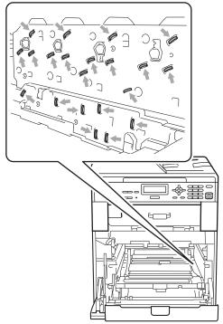
Hold the green handles of the drum unit when you carry it. DO NOT hold the side of the drum unit. Hold the handle of the toner cartridge and slightly push it to unlock it. Then pull it out of the drum unit. Repeat this for all the toner cartridges.
