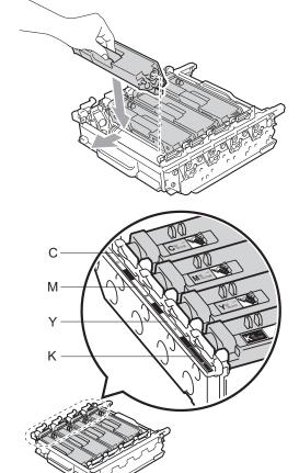
C - Cyan M - Magenta Y - Yellow K - Black 8 Make sure the green lock lever (1) is in the release position as shown in the illustration.
