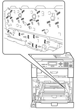
Hold the green handles of the drum unit when you carry it. DO NOT hold the side of the drum unit. Wipe the four scanner windows (1) with a dry, lint-free cloth.
