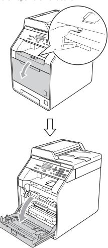
4 Hold the green handle of the drum unit. Pull the drum unit out until it stops.
