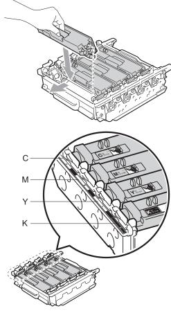
C - Cyan M - Magenta Y - Yellow K - Black Make sure the green lock lever (1) is in the release position as shown in the illustration.
