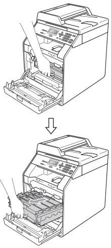
Turn the green lock lever (1) at the left of the machine anticlockwise to the release position. Holding the green handles of the drum unit, lift the front of the drum unit and remove it from the machine.
