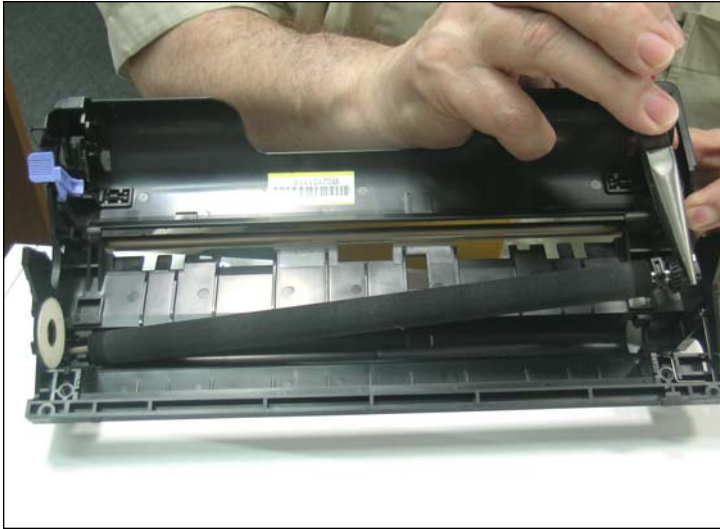
26. Replace the transfer roller together with its saddles and the helical gear.
