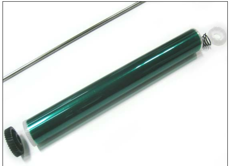
23. Do not lose these three pieces which will be needed to assemble the cartridge even if a new drum is installed.
