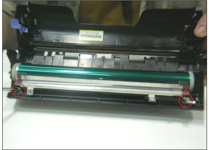
17. With a Phillips screwdriver remove the screws holding the drum cleaning assembly. You will notice that it is composed of a cleaning felt, a recovery blade and a couple of scraper-blades.
