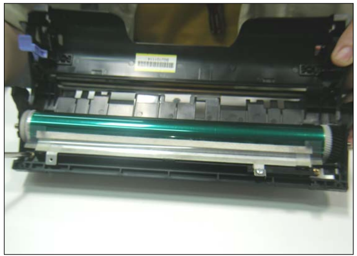
29. Insert the drum cleaning assembly and with a Phillips screwdriver and tighten the screws to secure it to the cartridge. The screw on the left will pressure the contact between the assembly and the drum axle.
