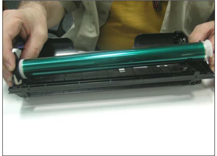
27. Replace the OPC drum by mounting the clutch and spring on the right side and engage the drive gear on the left. NOTE: Before inserting the axle lift the spring loaded contact wire located between the drive gear of the OPC and the side of the cartridge.
