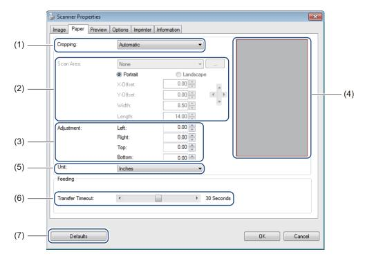
Cropping allows you to capture a portion of the scanned document.
