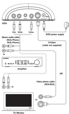
The iD50's audio outputs can be connected to a stereo system or suitable TV with audio inputs and built-in amplification as shown above. For the best quality, we recommend use of a good quality hi-fi separates system.
