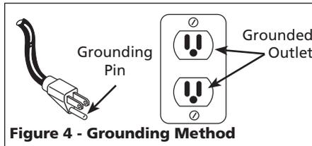
Figure 4 - Grounding Method
