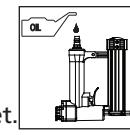
Do not use detergent oils, oil additives, or air-tool oils. Air tool oils contain solvents which will damage the tool's internal components.
