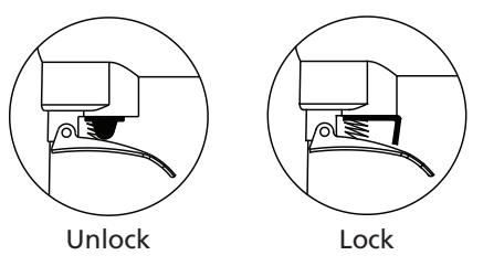
After verifying there are no fasteners in the tool, safety check the operation of the activated trigger lock to prevent the tool from firing a fastener before storage. Always disconnect from compressed air when not in use.
