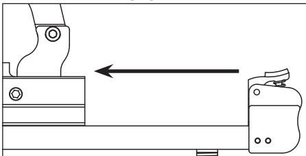
5. Always unload all fasteners before removing tool from service. Unloading is the reverse of loading, except always disconnect the air supply before unloading.
