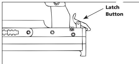
3. Insert a stick of fasteners into the magazine with pins positioned as shown. Make sure pins are not dirty or damaged. Pins are marked for direction of loading.
