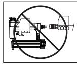
**WARNING** Always disconnect the tool from the power source when unattended, performing any maintenance or repair, clearing a jam, or moving the tool to a new location. Do not load the tool with fasteners when the trigger is depressed. The tool could eject a fastener causing death or serious personal injury.
