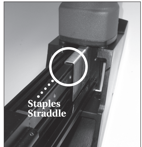
Figure 17 - Place STAPLES straddling the top of the magazine
