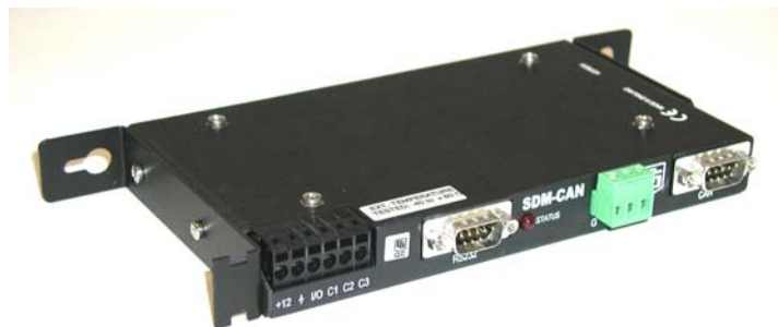
Figure 1-1 SDM-CAN CAN-Bus Interface
