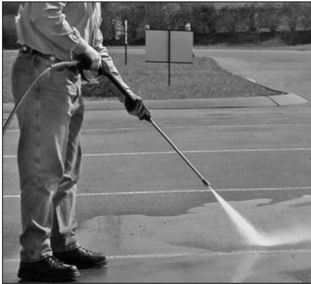
Figure 11 - Optimum angle to cleaning surface
