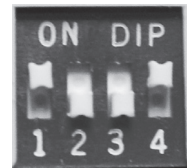
DIP SWITCHES SET TO '1001'
