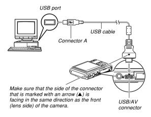
Take care when connecting the USB cable to the camera or your computer. USB ports and cable plugs are shaped for proper positioning.
