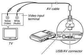
Make sure that the side of the connector that is marked with an arrow (**A**) is facing in the same direction as the front (lens side) of the camera.
