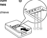
[CHARGE] lamp lights red during charging. [CHARGE] lamp goes out when charging is complete.
