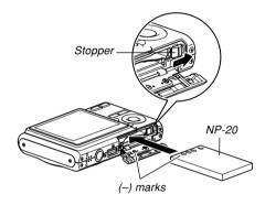
• Push the bottom of the battery, and make sure that the stopper securely locks the battery in place.
