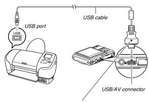
Make sure that the side of the connector that is marked with an arrow ( $\Delta$ ) is facing in the same direction as the front (lens side) of the camera.
